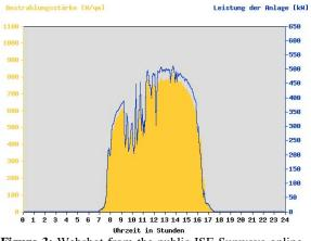
**Figure 3:** Webshot from the public ISE Sunways online monitoring portal showing the solar irradiance characteristics in the tracked module plane (left axis W/m2) together with the AC power feed into the grid (right axis kW) at the 19<sup>th</sup> of Oct 2009.[4]
