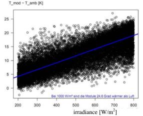
**Figure 4:** Measured temperature difference between PV modules and ambient temperature versus irradiance [W/m<sup>2</sup>] during 2009 (average module temperature during day time was 25.1°C and average ambient temp 11.2°C [4]
