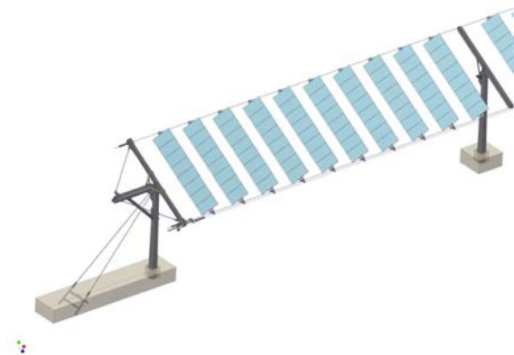
Figure 12: Concept of the first Solar Wings two-axis tracking system. The first prototype with 70kW nominal power will be installed in Nov 2009 in Switzerland
