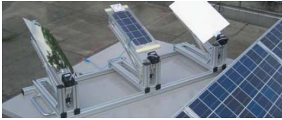
Figure 8: Experimental setup to measure the power gain of low-concentration using parallel tracking axis.
