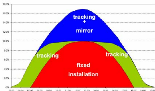
Figure 12: Typical characteristics of solar input during the course of a day of classical tracking and individually tracking of PV modules and mirrors to reach low-concentration (latitude 47° north, all tracking axis are parallel).
